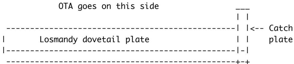
The catch plate has cutouts at its bottom corners to clear the grooves on the dovetail plate -- you can slide the dovetail plate into the dovetail plate clamp even with the catch plate attached. That's important, because the bolts that hold the tube ring to the other end of the dovetail plate prevent you from sliding the dovetail plate into
