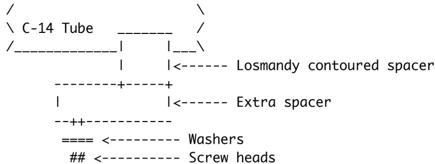
The Losmandy dovetail plate has a big wide groove milled down its center line, on the side toward the OTA. The screws and washers loosely engage that groove, so as to provide lateral guidance for the cell end of the telescope as I settle the whole thing down into the dovetail-plate-with-tube-ring. And there is still more:
